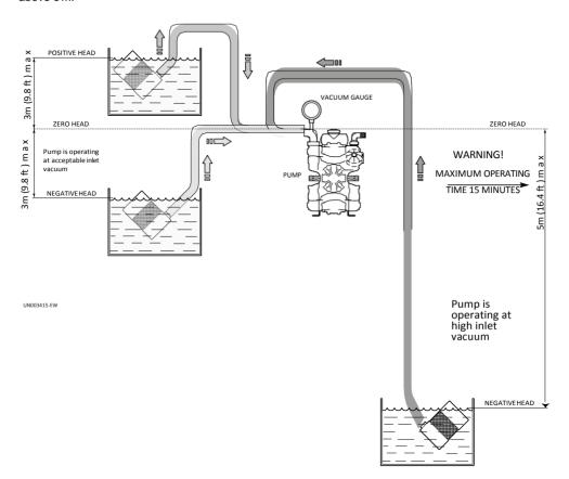
For continuous duty, the pump should not draw in liquids by vacuum from containers with the liquid level more than 3 m below the pump intake fitting and the circuit must consist of hoses of length and diameter appropriate to the pump intake fitting (see "Technical Data"), free from restrictions and elbows, and with a filter of suitable capacity (see "Installation").
